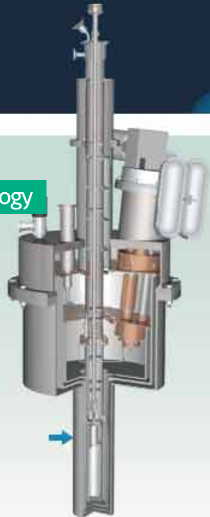
▲ Cryogen free top-loading cryostat based on a pulse-tube refrigerator. The arrow indicates the height of the beam.
