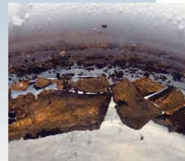
▲ Metallic \text{Li}(\text{NH}_3)_4 photographed in liquid nitrogen in the open lab. This ultra-light bronze metal even floats!
