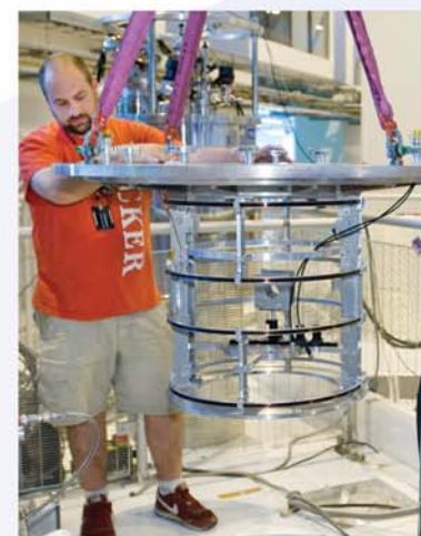
Stephen Boag (ISIS) craning the polarisation field-coil insert into the Wish diffractometer.
