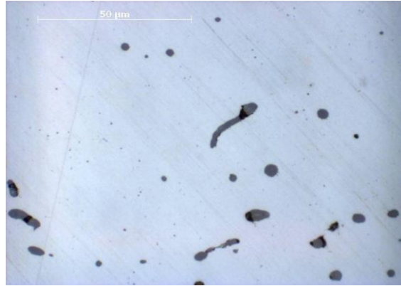
Figure 2.7. Micrograph of MnS inclusions in steel matrix of a free cutting steel studied in this thesis.
