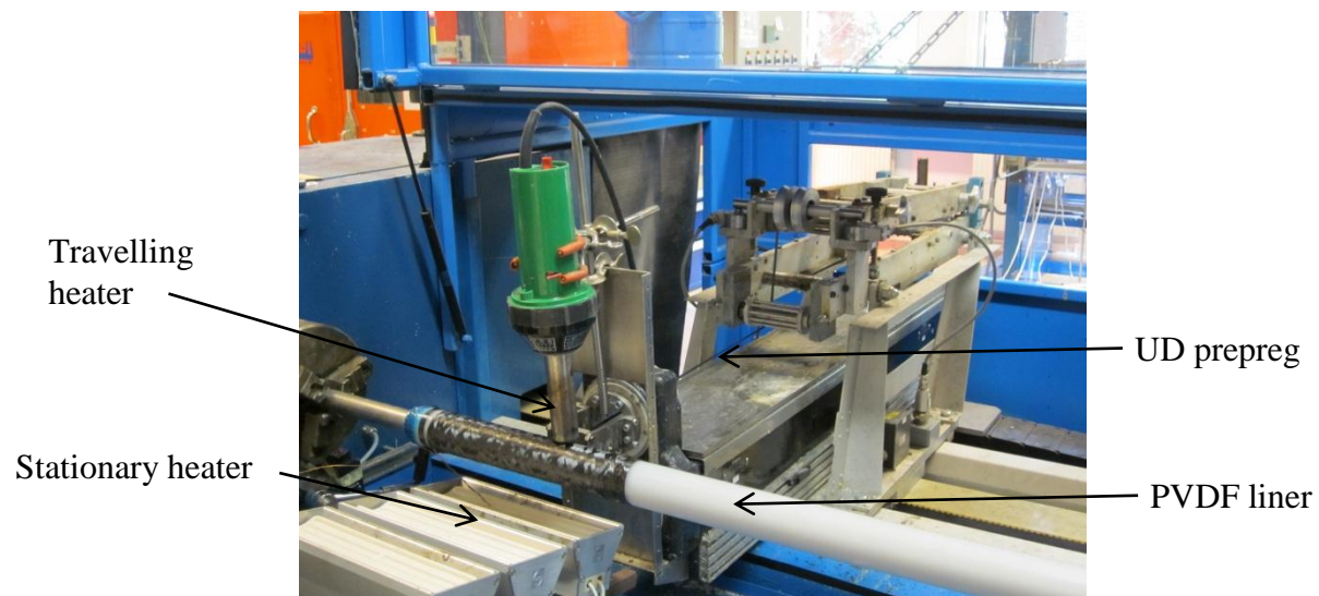
Figure 7.1 Photographic image of filament winding unit used to fabricate reinforced thermoplastic pipe
