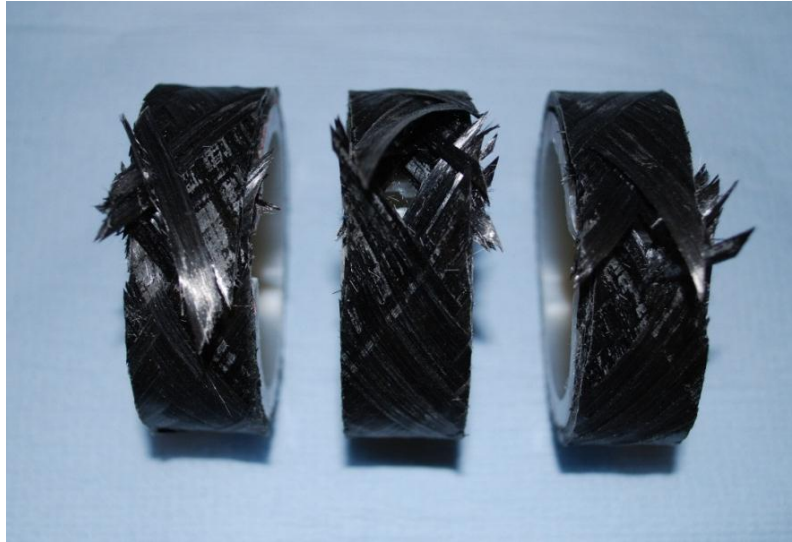
Figure 7.4 RTP consisting of a PVDF liner reinforced with layers of \pm 55^\circ carbon fibre reinforced PVDF after subjected to split disk tensile test
