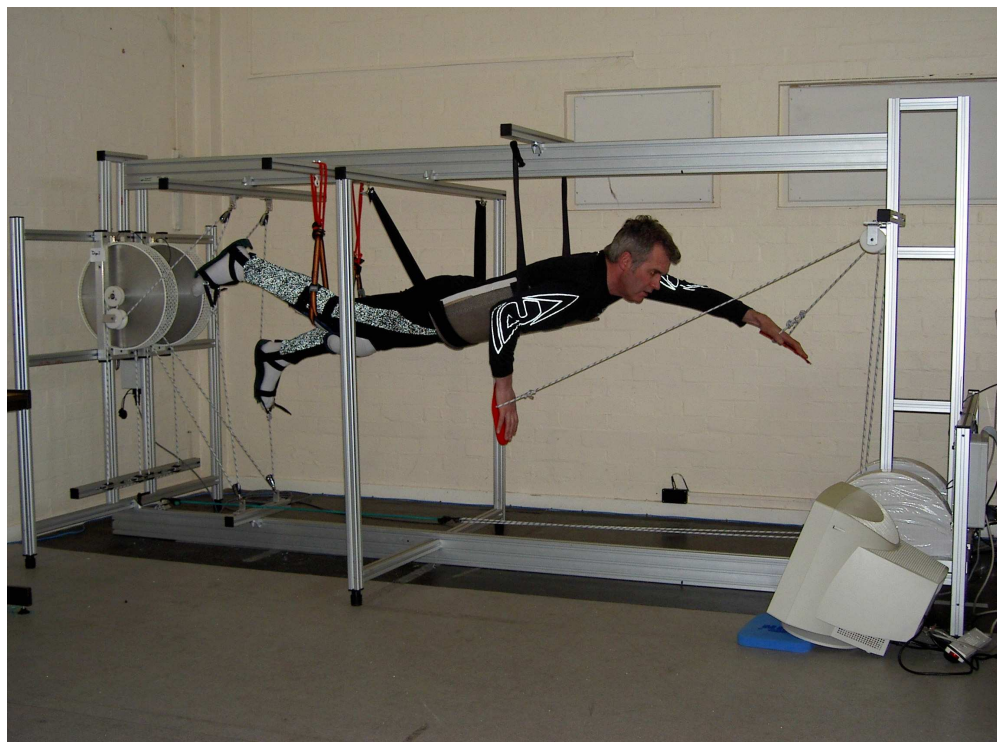
Figure 1. Photograph of the novel swimming training machine. 609x450mm (96 x 96 DPI)
