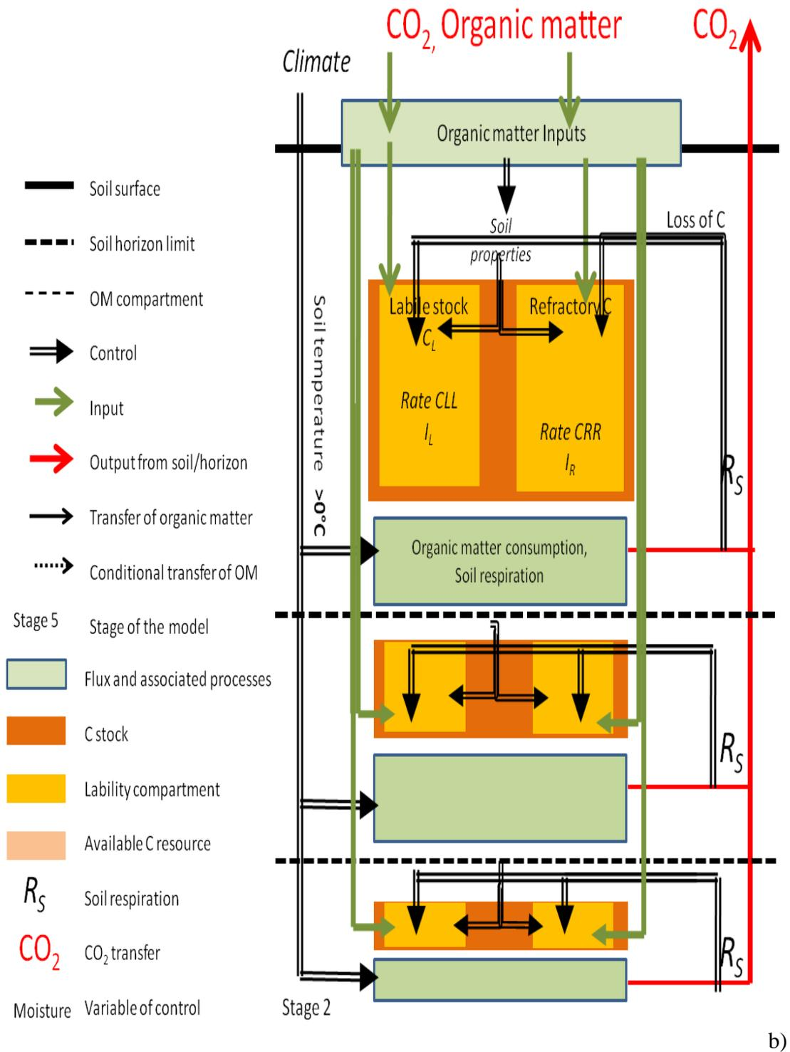
**Figure 4.2 b: Stage 2 structure with several soil horizons; the inputs of  $CO_2$  and organic matter going into the soil and ending up either in the labile or recalcitrant C compartment; the respiration rate is only function of the temperature; variables are explained in Appendix A4.1**
