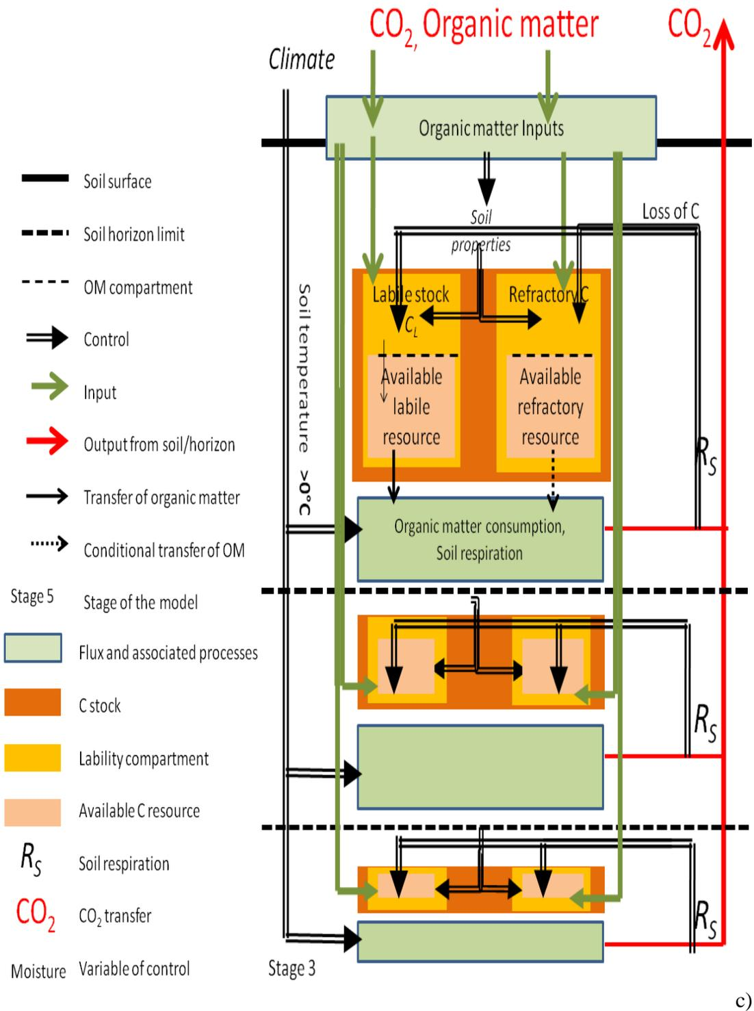
**Figure 4.2 c: Stage 3 structure with several soil horizons; the inputs of CO<sub>2</sub> and organic matter going into the soil and ending up either in the labile or recalcitrant C compartment; the respiration rate is only function of the temperature and can use the stocks of labile C; variables are explained in Appendix A4.1**
