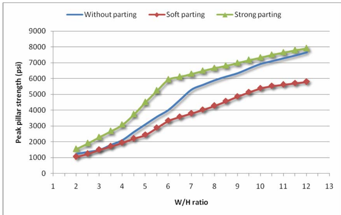
Figure 9: The effect of the parting on coal pillar strength in FDM modeling
