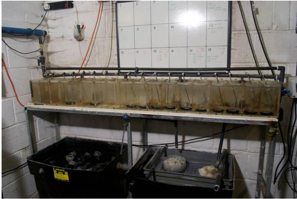
Figure 2. 1 Freshwater, down-welling incubation system in the Tropical Aquarium, University of Stirling.
