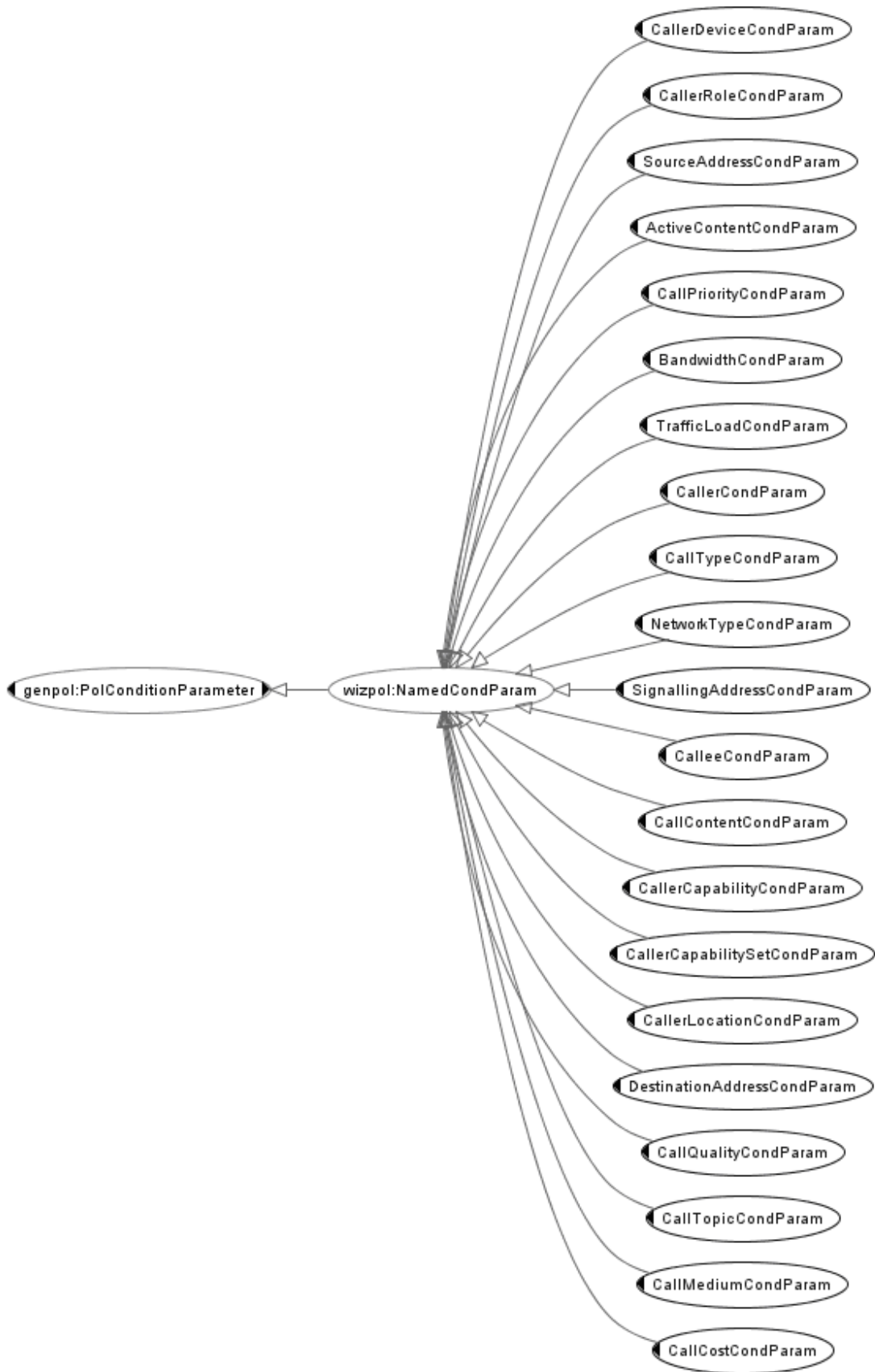
Figure 4.14: Telephony Named Condition Parameters
