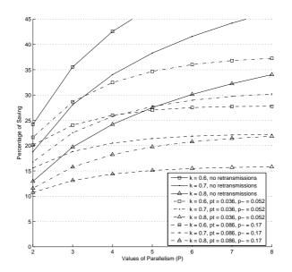
Figure 5.19: Saving achieved using XCAST for varying factor k. [9] and pt = 0.086 and p-=0.17 (churn intensive), and k = 0.7 the saving is about 22%. This matches our simulation results and proves that significant savings can be achieved overlay operations using XCAST.
