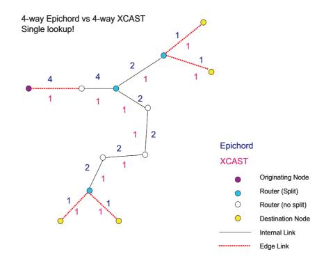
Figure 5.2: Progress of a multi-destination multicast message through a network
