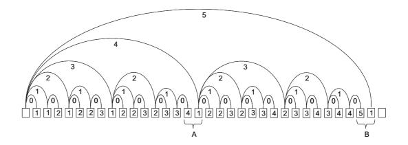
Figure 6.1: Propagation delay for a single event for different paths. Adjacent nodes at A receive messages at intervals 4 and 1 while adjacent nodes B are intervals 5 and 1. [12]
