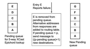
Figure 5.12: Failure scenario for a 5-way XCAST EpiChord request.
