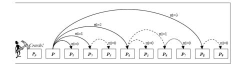
Figure 4.5: A D1HT system with 11 peers (p = 4), where a peer crashes and this event is detected and reported by its successor nodes. Each peer should only receive one single notification of the event [7].
