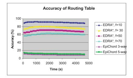
Figure 6.3: Routing table accuracy of EDRA<sup>\*</sup> over varying degrees of f and EpiChord over varying degrees of parallelism [12]
