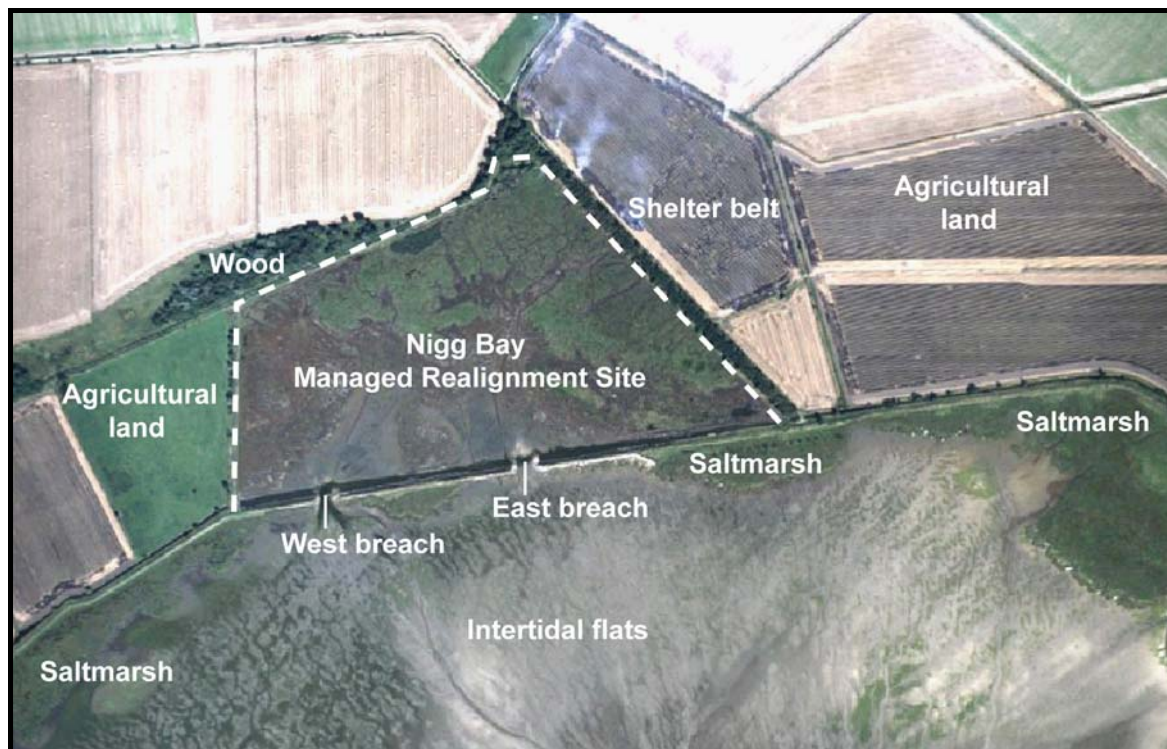
Figure 2.7: Nigg Bay Managed Realignment Site. Aerial photograph taken in September 2003, seven months after the reintroduction of tidal conditions. The dashed line indicates the secondary defence. NERC ARSF.
