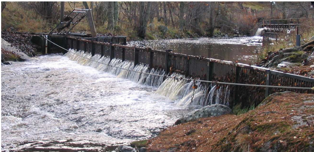
Figure 2.3 The upstream trap at Girnock Burn. The holding cage is visible on the far left hand side of the figure. The downstream trap is just visible in the top right hand corner.
