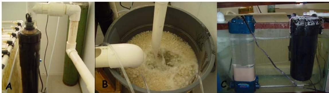
Figure 5.8. Microcosm filtration system, A) UV light, B) bio-filtration beads C) Fluidised bed and Carbon filter (right)
