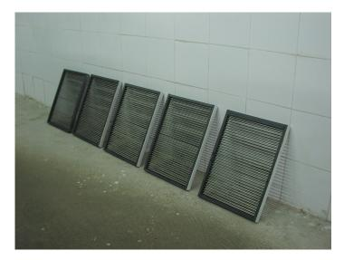
Figure 5.1: Grading sheets designed for the experimental grading of gilthead seabream juveniles. The 5mm stainless steel bars are fitted into a plastic collar by holes drilled at fixed widths. The sheets are then slotted into a fibre-glass box which holds the sheets 10cm under the water's surface. Gap sizes of the sheets were 1.5, 2.0,2.5, 3.0 and 4.0mm; accurate to 0.1mm.
