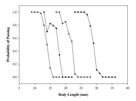
**Figure 5.3:** Performance of farm grading sheets. Probability of a given body length passing through each grading sheet based on 100 measurements per sheet from post-graded groups. Grader sizes: 1.5 mm (---), 2.0 mm (---), 2.5 mm (---), 3.0 mm (---) and 3.5 mm (---).
