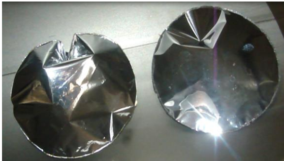
Figure 5. Circular prototypes inflating under vacuum conditions
