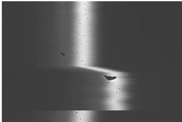
Figure 6 Tilted mirror test for optical sectioning in confocal reflection mode. If a known vertical shift of focus can be imposed ( 5 \mu\text{m} in this case) the mirror gradient along a horizontal line in the figure can be deduced.
