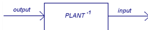
Figure 3 – Inverse Dynamics; the Control System calculates the input required for a desired output
