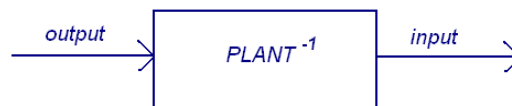
Figure 3 – Inverse Dynamics; the Control System calculates the input required for a desired input
