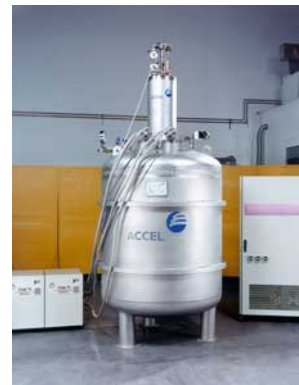
Figure 7-1 2MJ, 200kVA (8 second carry-over time) SMES system
