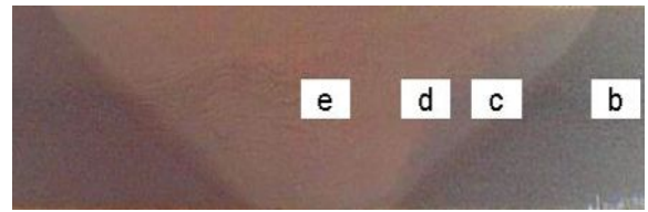
(a) macrostructure of the single sided FSWd plates
