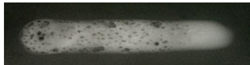
Fig. 2b: An X-Ray image of a highly porous weld
