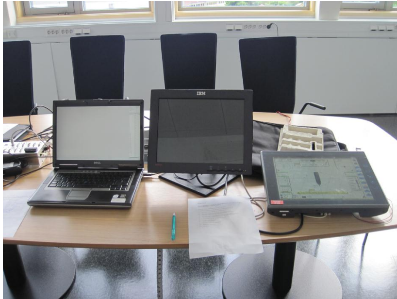
Figure 11: Control laptop, NextWindow multi-touch display, Single touch DP display
