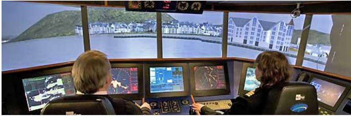
Figure 13: Motion simulator with visualisation of environment
