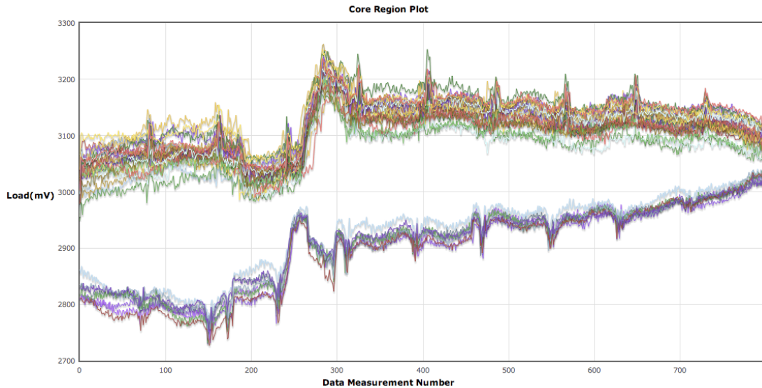
Figure 2. Plot showing multiple FGLT traces on the same graph, illustrating the repeatability of the response between different events
