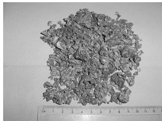
Figure 10: Appearance of recovered stainless steel.
