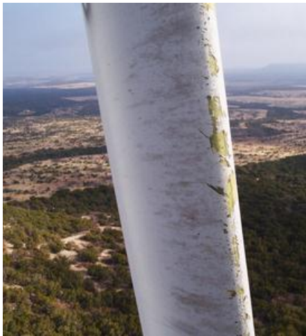
Figure 2. LEADING EDGE EROSION (presented without scale), SOURCE: [7]
