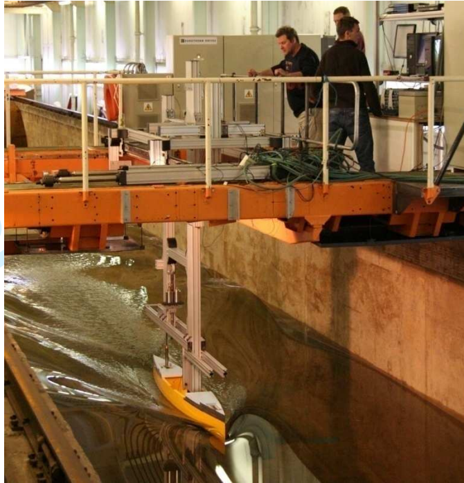
Figure 4 Shallow water testing of Wigley Hull
