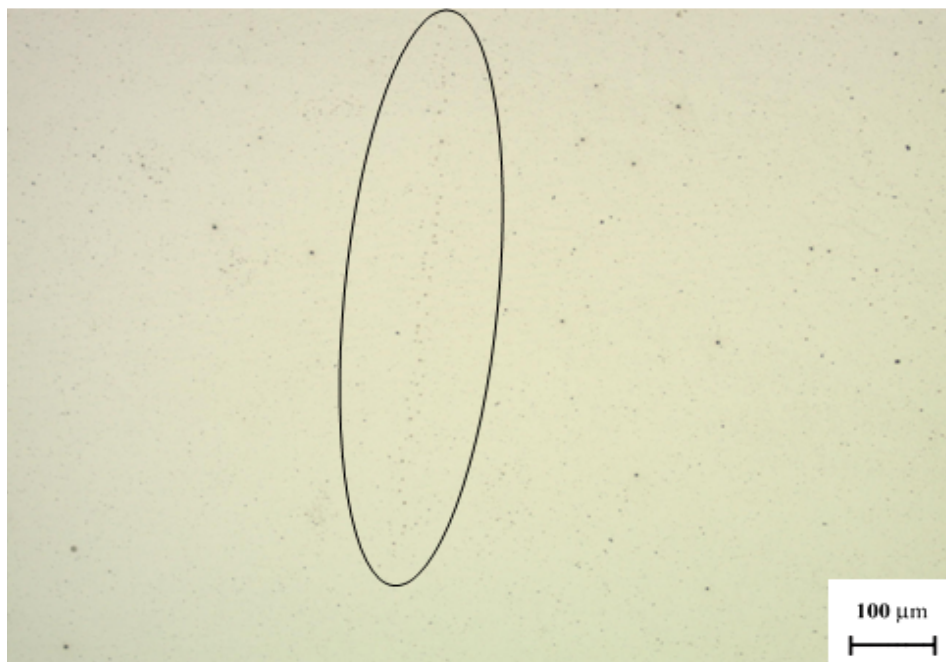
Figure 2: Weld micrograph produced using electromagnetic gas saving device showing fine line of impurities
