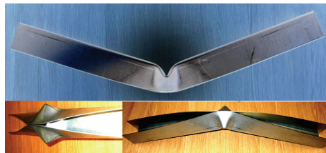
Figure 3: U-section collapse mode for all impact velocities
