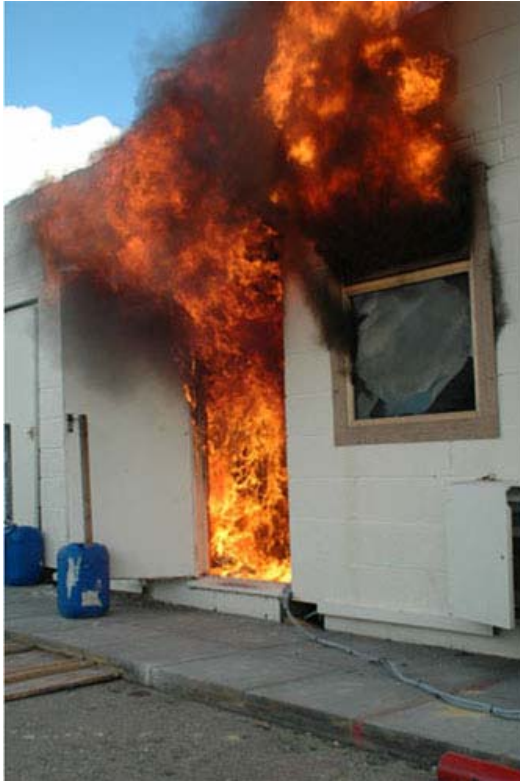
Figure 1 – a view of an experiment fire during flashover conditions.
