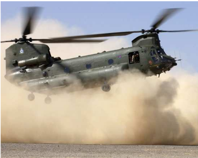
Figure 1: Chinook helicopter landing in dusty conditions. Note the cloud of dust that is being produced below the aircraft; brownout is a distinct possibility should the aircraft decelerate or descend. (Image Crown copyright.)
