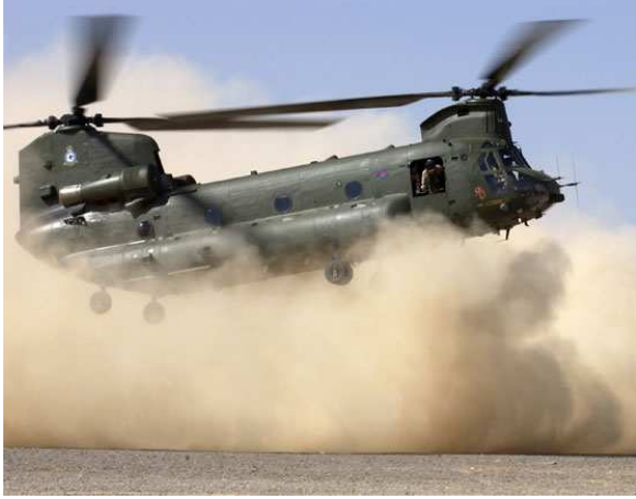
Figure 1: Chinook helicopter landing in dusty conditions. Note the cloud of dust that is being produced below the aircraft; brownout is a distinct possibility should the aircraft decelerate or descend. Image courtesy UK MoD.
