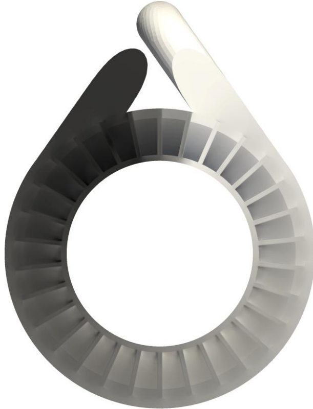
Figure 8: Tangential pressure rise through axial regenerative pump
