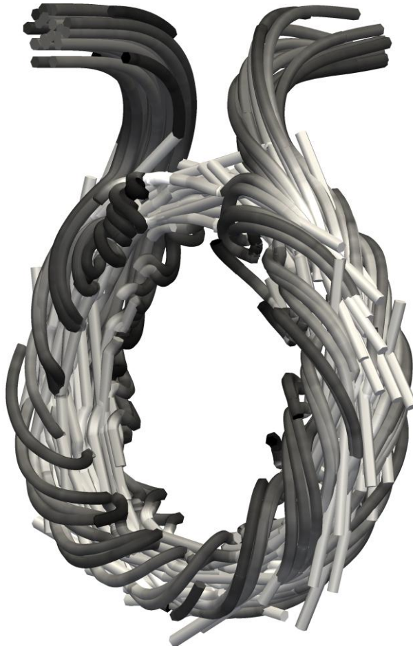
Figure 6: Regenerative Pump helicity pathlines plot
