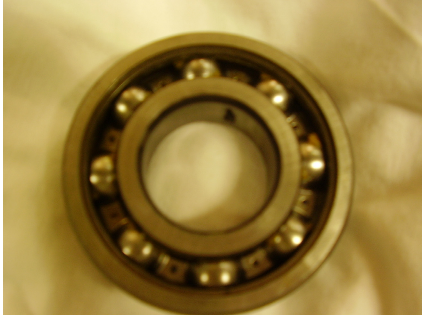
Figure 4. Bearing with an inner race fault
