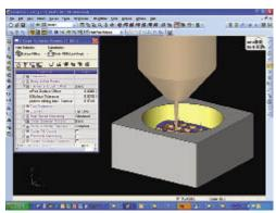
Software developer Cimatron says its CimatronE Micro Milling CAM software can create toolpaths capable of producing tolerances as tight as 0.000004", using cutting tools as small as 0.004" in diameter and smaller and running at 150,000 rpm or faster. Image courtesy Cimatron.
