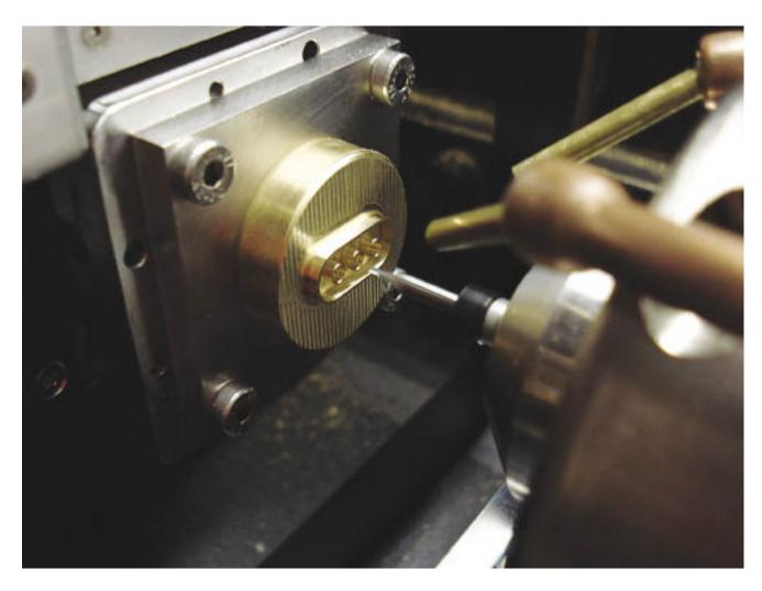
As milling tools shrink in diameter, a number of factors loom large in generating fine surface finishes. Photo courtesy Microlution.
