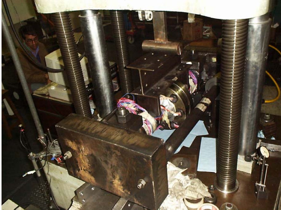
Plate 1 Standard, gasketed joint under combined loading
