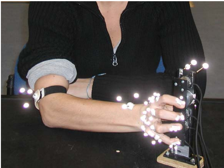
Figure 2. Subject performing the force experiment with the wrist in a functional neutral position. Motion capture markers are attached to the arm, hand and force measurement device.
