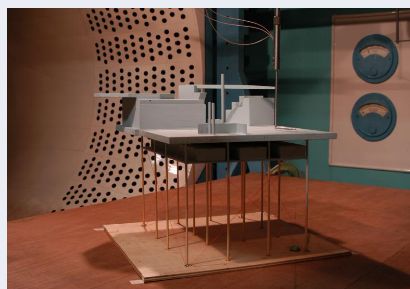
Figure 2; Low speed wind tunnel model.
