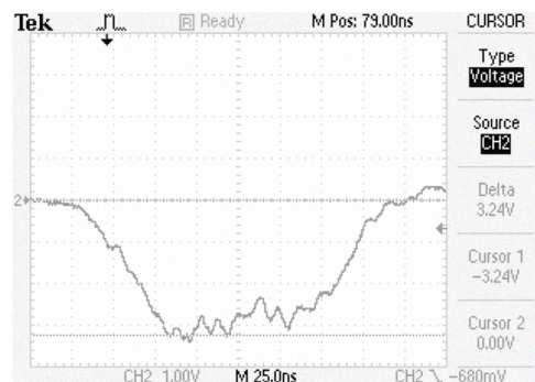
Fig. 3. Trigger pulse voltage waveform from Blumlein. The magnitude is ~75 kV, the pulse width is 125 ns, and the rise-time is 50 ns.
