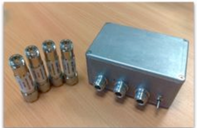
Figure 3. A Low-power 3-channel detector with externally mounted band filters.
