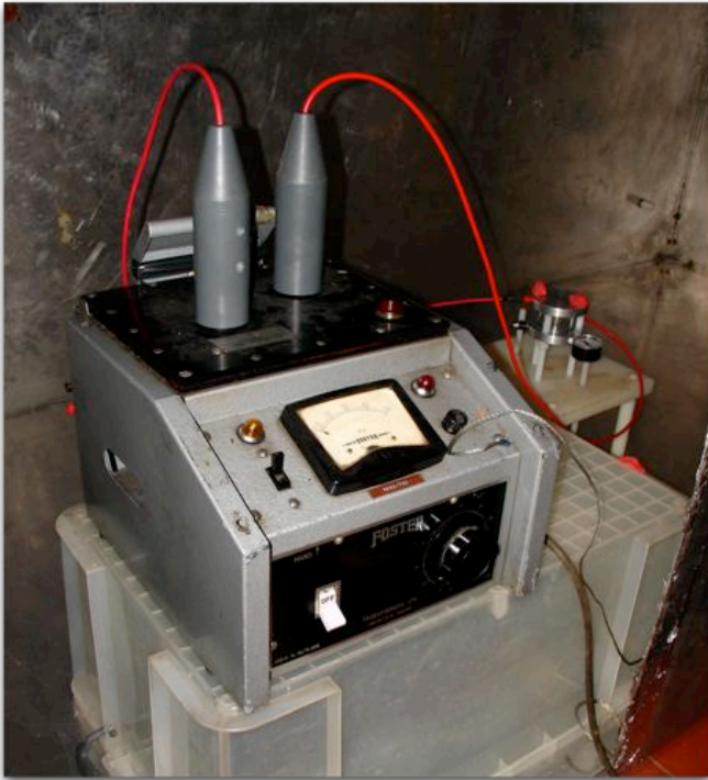
Figure 7. Internal view of RF test tank, with 50kV transformer. The rolling particle in SF 6 test cell can be seen behind.
