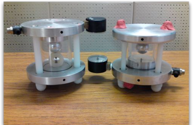
Figure 6. Two of the test cells used for the experiment. On the left is the floating electrode in SF 6 test cell, and on the right is the rolling particle in SF 6 test cell. The cells are approximately 15cm tall.
