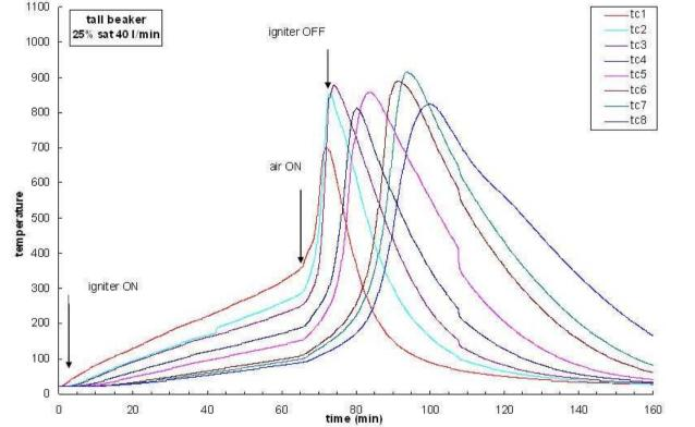
Temperature profiles, as measured by thermocouples embedded in the contaminated soil and the clean sand above, are typical of smouldering but the observed temperatures are significantly higher.
