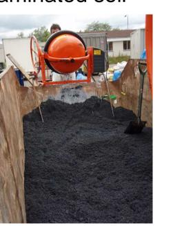
Mechanically mixed coal tar in sand or field-obtained contaminated soil
