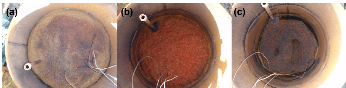
Figure 3. Excavation of the prototype field experiments revealed a variety of materials that corresponded well to observed temperature profiles. (a) Incomplete smouldering was observed at the top of the clean sand cap, (b) cleaned sand was observed through the majority of the sand pack and (c) a cone of charred coal tar in sand with two channels of clean sand was observed in the 20cm space above the igniters.
