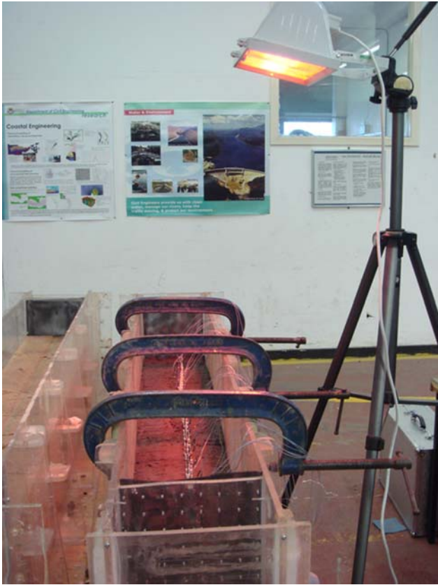
Fig. 2 Experimental setup with infra-red heater and electrodes installed
