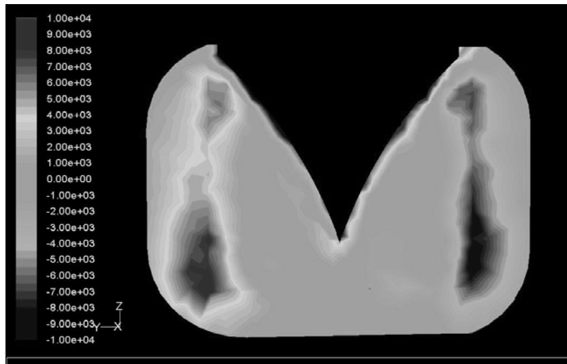
FIGURE 12. Regenerative Pump Helicity Contours
