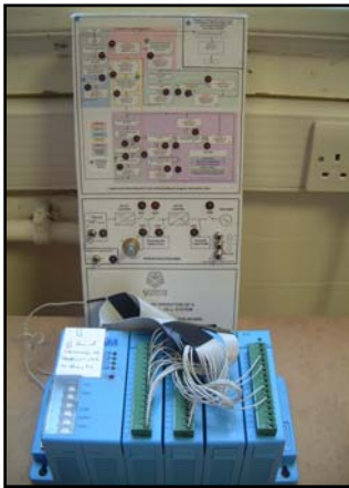
Figure 8(a). FC/battery hybrid system emulator.
