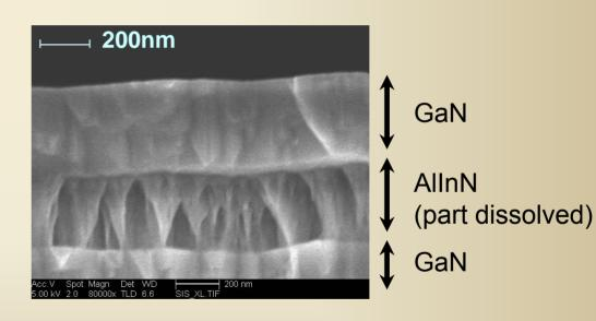
The 300nm AllnN layer has been undercut and etched into conical forms
