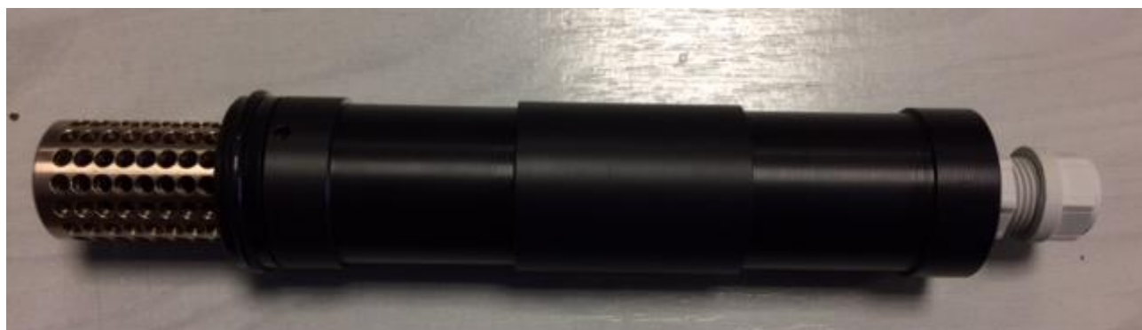
Figure 3: Picture of the novel SSS sensor, which actually measures temperature and conductivity.
