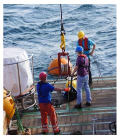
5 moorings with ADCP's and T, S, O<sub>2</sub> recorders
