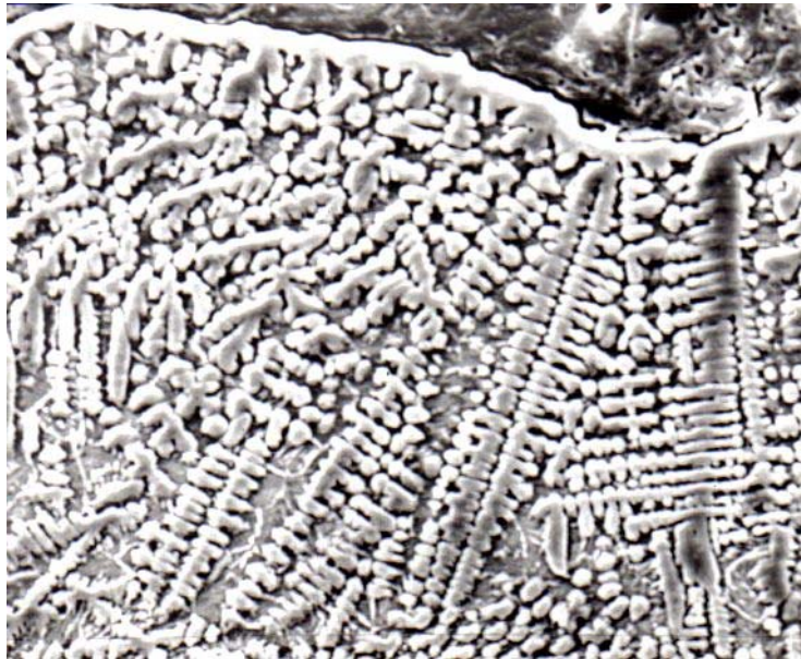
18.12 Heterogeneous distribution of dendrites following laser nitriding (Mridha and Baker 1996) Page 11
