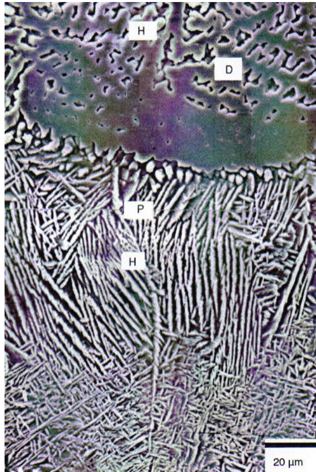
18. 15 SEM micrograph of laser processed SiC preplaced powder on CPTi, showing small needles(10-15 \mu\text{m} )below larger needles (30-35 \mu\text{m} ) following a concentrated dendritic structure(D).Platelet particles(P) in the needle structures and variation of the hardness indentations(H) are also visible (Mridha and Baker 2007).
