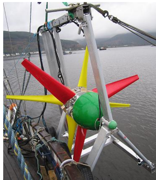
Figure 1: 2.5m diameter contra-rotating Marine Turbine (CoRMaT)
