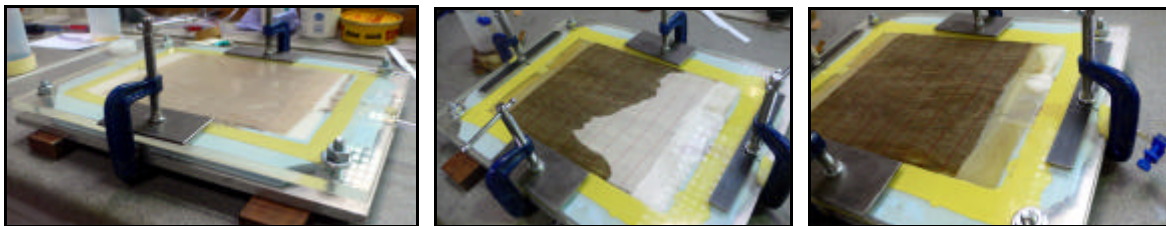
Fig. 1: left to right. The vacuum infusion rig, mould during infusion, and rig just after fill
