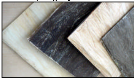
Fig. 2: Composite materials manufactured in plates by vacuum infusion (approx 60% Vf)
